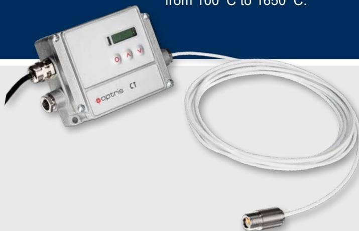
The infrared thermometer optris® CTlaser G5 allows for temperature measurement of **smallest objects of 1 mm** from a distance of 70 mm. Due to its **very short response time** of 10 ms it is often used for fast processes.
