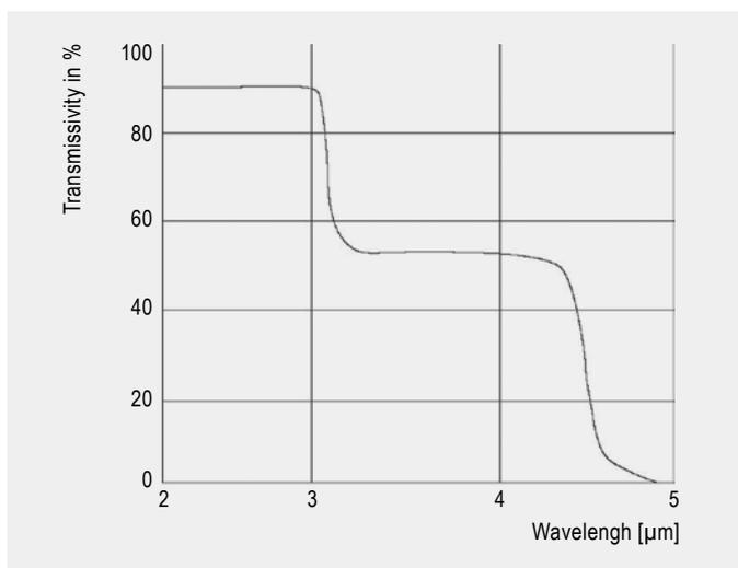
Spectral transmissivity of glass
